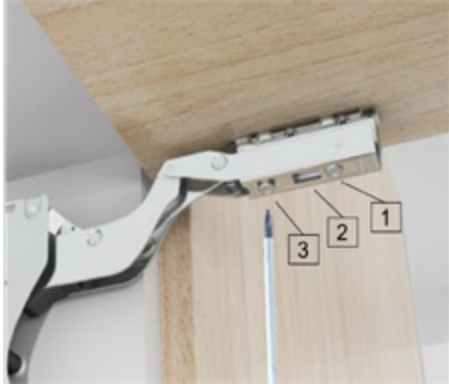
Panel can make 3D adjustment Adjustment range: 1.Up&Down 2.Left&Right 3.Front&Back
